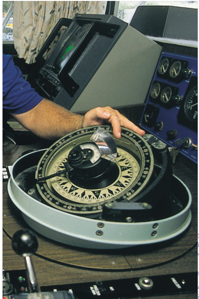
Figure 15.1 Binnacle mounted compass. Note — A binnacle is the pedestal in which a compass is mounted.
