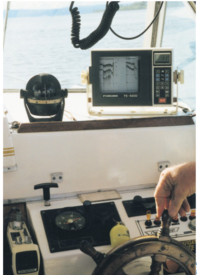
Figure 28.1 Depth sounder mounted in wheelhouse of small boat. (Photo Courtesy Dave Claridge)
