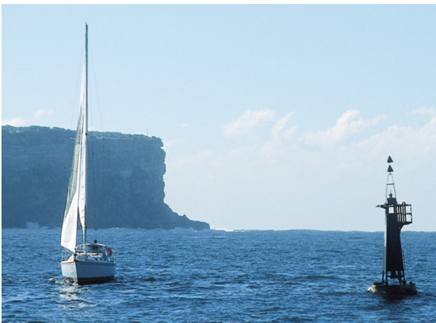
Figure 42.3 A fixed mark is used to swing a compass on a small vessel.
